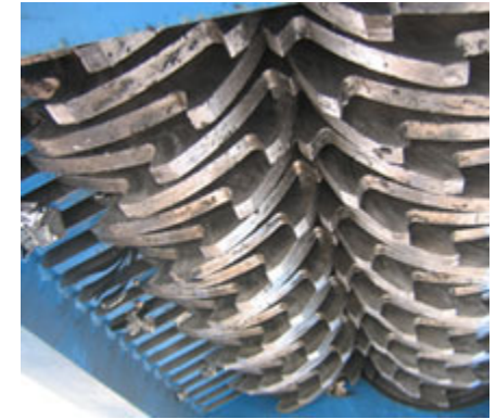
Shredding chamber discharge side shows rugged cutters
